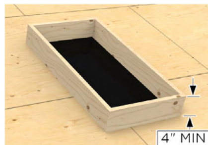
Wood-framed curb around skylight penetration.
