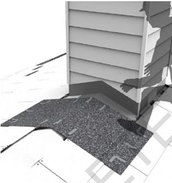
Pictured: Example of traction mats used at low slope at a ridge obstruction.
